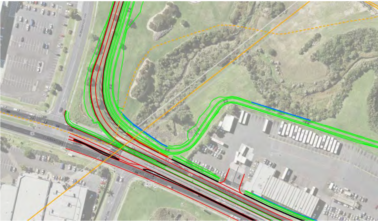
Figure 10 – High Voltage Transmission Plan at Burswood Reserve (overhead line is solid orange line, underground line is dashed orange line)
