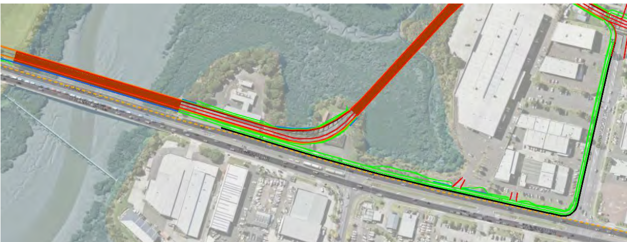
Figure 11 - High Voltage Transmission Plan at China Town (underground line is dashed orange line)
